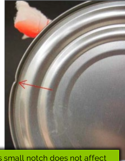
This small notch does not affect the integrity of the seam. It is safe!
